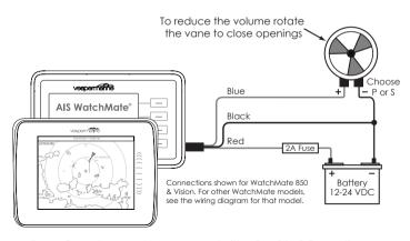
To configure the sound type, connect either P or S to DC negative. Do not connect both. Choose either P for pulse or S for steady sound.
